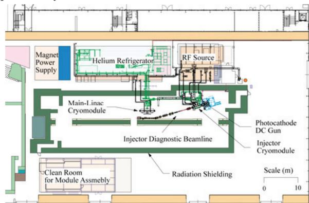
Figure 6: Layout of cERL in May, 2013. An injector has been completed and commissioned.
