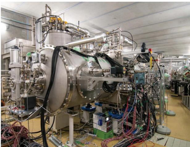
Figure 3: A cryomodule for the main linac.
