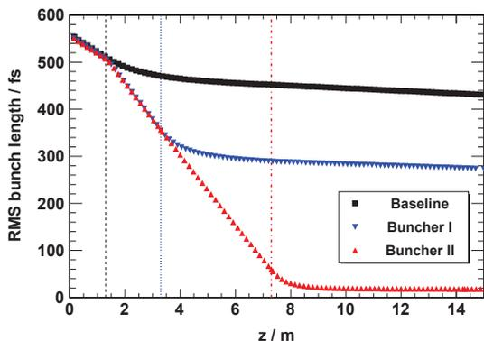
Figure 2: RMS bunch length evolution along the machine with deactivated magnetic bunch compressor simulated with ASTRA for the baseline design and the two buncher options. The vertical lines indicate the linac entrance in the different scenarios.
