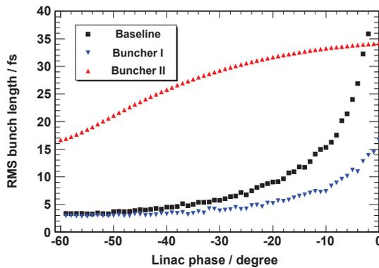
Figure 4: Compressed RMS bunch length vs. the linac phase using a peak E-field of 15 MV/m. Far off-crest there is no difference between the baseline and Buncher I.
