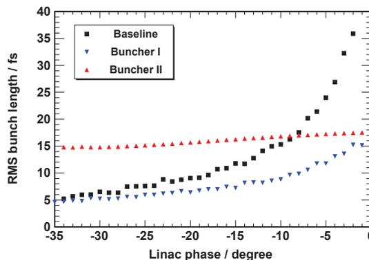
Figure 3: Compressed RMS bunch length vs. the linac phase using a peak E-field of 10 MV/m. Far off-crest there is no difference between the baseline and Buncher I. Buncher II shows higher values for all phases.
