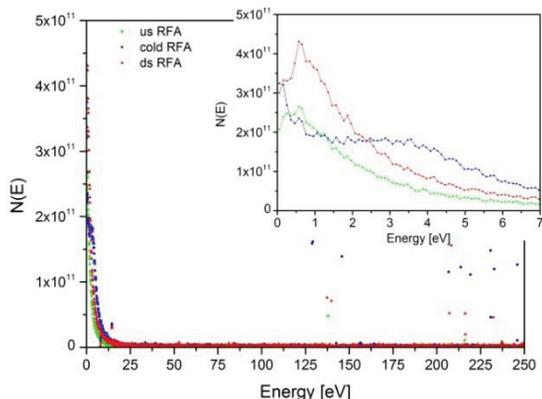
Figure 4: Energy spectrum from the three RFAs located upstream (us), downstream (ds) and in the cold section of COLDDIAG for 686 bunches and 300 mA beam current.
