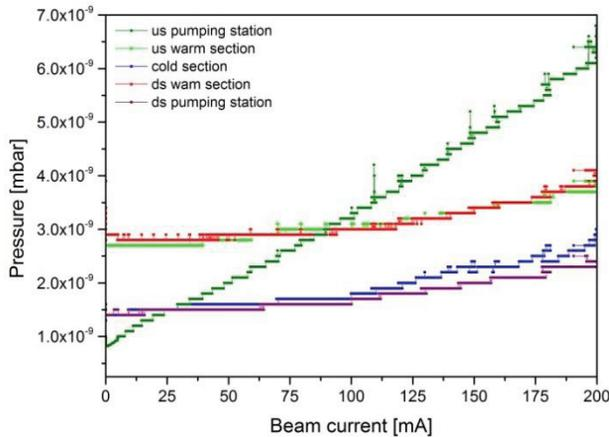
Figure 2: Pressure plotted against the average beam current for a filling pattern of 460 sequential bunches.
