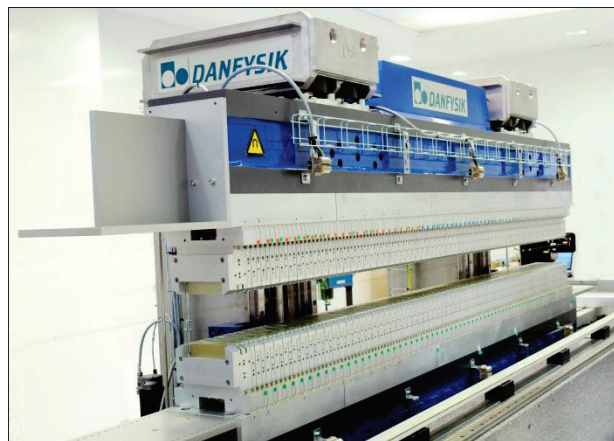
Figure 8: Damping wiggler for NSLS-II being shimmed.
