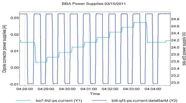
Figure 3: The power supply currents of a quadrupole (bi8-qt3) and a dipole corrector (bo7-th2) during BBA measurement with the typical procedure used before RHIC 2012 run.
