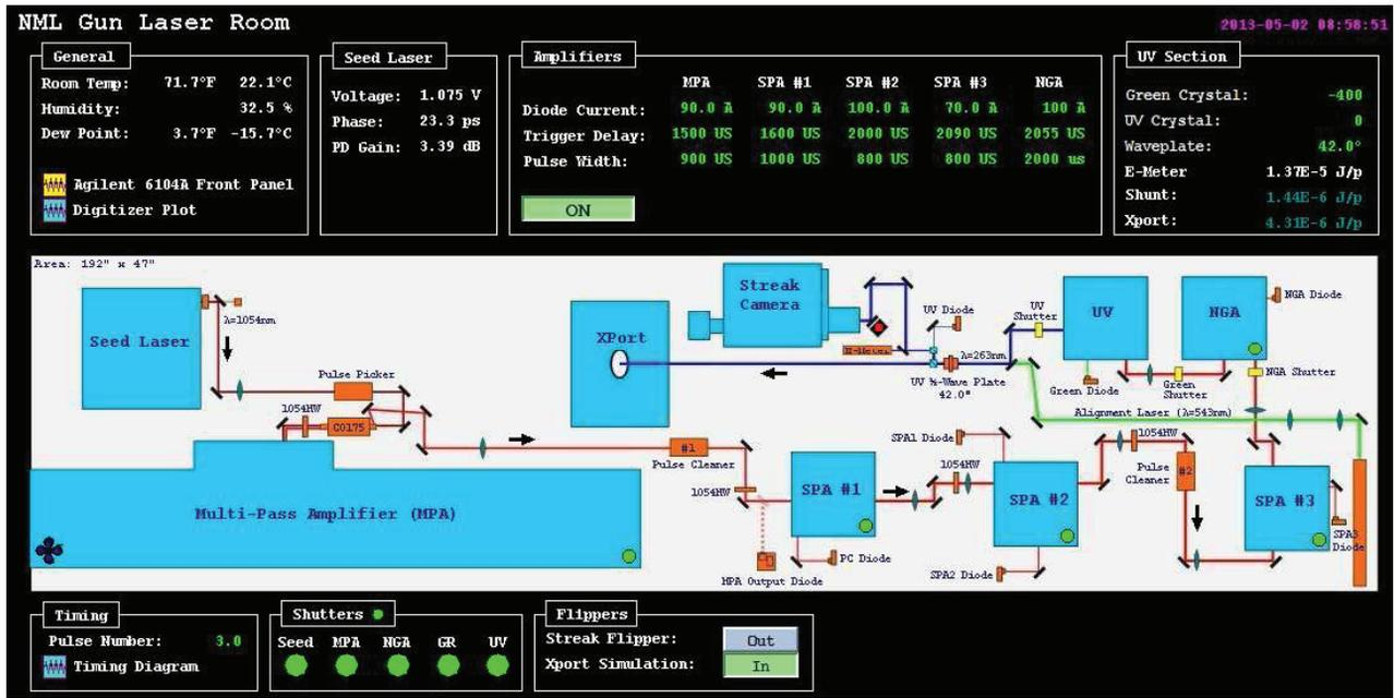
Figure 2: Synoptic user display of the NML Gun Laser system.
