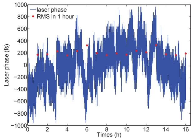
Figure 3: Laser phase measurement over a 16-hour period at steady-state. The blue line is laser phase while the red points represent the standard deviation of the laser phase noise over each hour.
