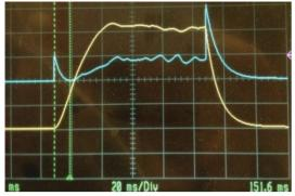
Figure 5: Cavity 1 open loop test, cavity driven by a rectangular pulse.
