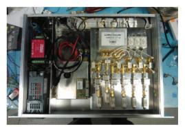
Figure 2: 19" enclosure, housing LLRF4 board and analogue components.
