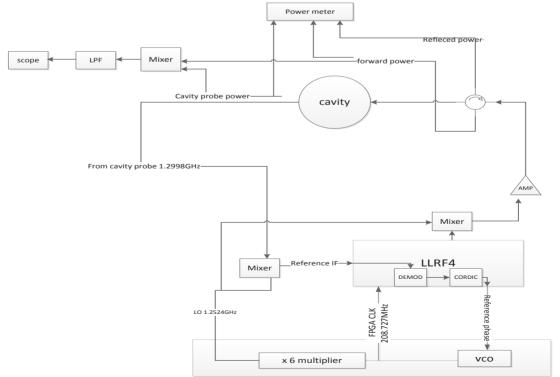
Figure 4: Digital VCO PLL system. LLRF4 board performs as a digital phase detector to regulate the VCO frequency.
