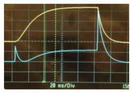
Figure 6: Cavity 1 closed loop test. Cavity controlled by digital self-excited loop. Signal noises are largely suppressed by the phase lock loop.
