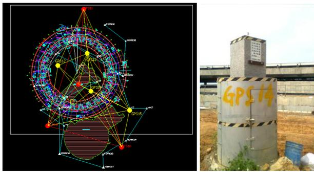
Figure 2: The GPS network of TPS
