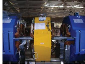
Figure 4: A foam tube coated with aluminum tube is introduced for eliminating air disturbance.
