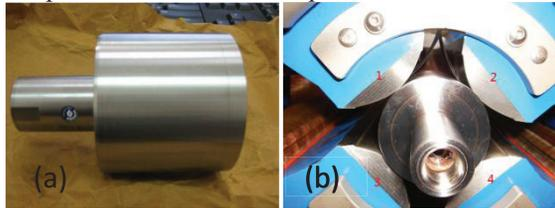
Figure 2: (a) Typical plot of the expansion mandrel (b) The expansion mandrel can be applied to insert into the quadrupole.
