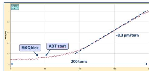
Figure 4: The root-mean-square of the orbit oscillations growing in time.
