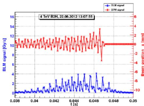
Figure 2: Comparison of BLM (blue line) and BPM (red line) signals (4 TeV).
