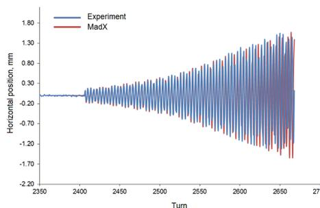
Figure 5: Comparison of MADX simulation and data collected during quench test.
