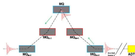
Figure 1: The concept of the quench test: a three-corrector orbit bump and beam excitation with ADT.
