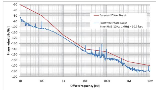
Figure 4: Required and achieved phase noise levels of 1300 MHz signal.
