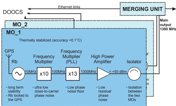
Figure 3: Master Oscillator system architecture.
