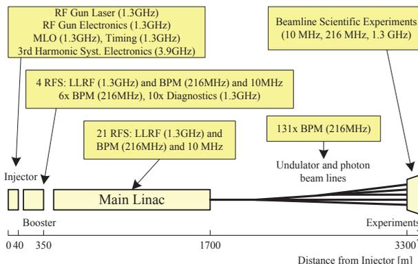
Figure 1: E-XFEL subsystems requiring RF phase reference signals.
