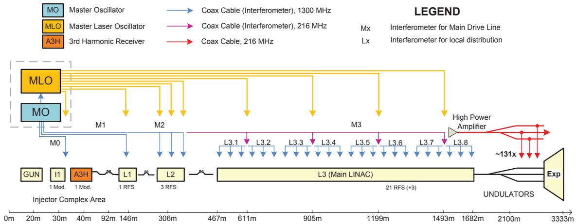
Figure 2: Simplified layout of the RF Phase Reference Distribution System in XFEL.
