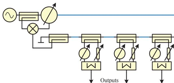
Figure 5: Conceptual diagram of interferometer link.
