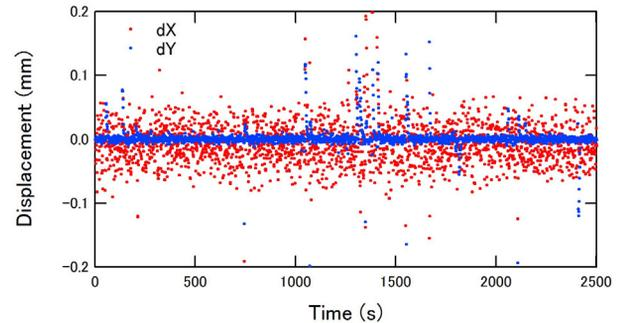
Figure 9: Time trend of the beam displacements at BPM #2 with the  $dY$  feedback control.
