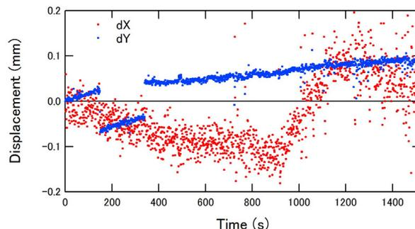
Figure 5: Time trend of the beam displacements at BPM #2.
