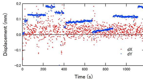
Figure 7: Time trend of the beam displacements at BPM #2 with the dX feedback control.
