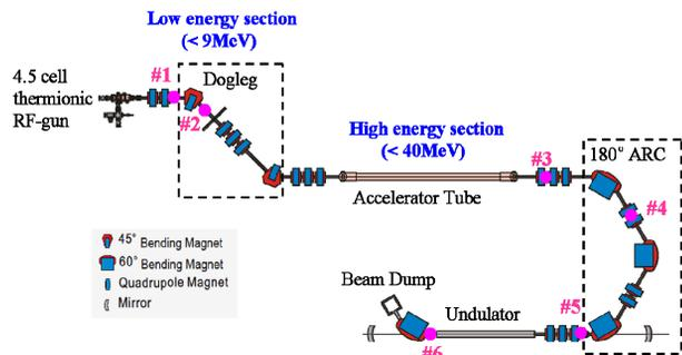
Figure 2: Layout of the KU-FEL driver linac. #1-#6 indicate the each position of BPM.
