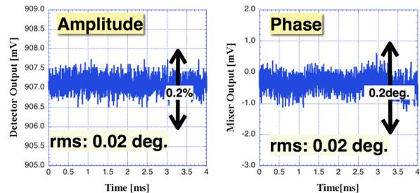
Figure 5: Short-term amplitude and phase stability under feedback control evaluated by out-of-loop measurement.
