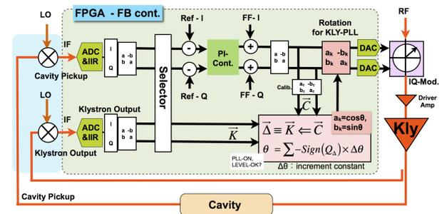
Figure 8: Design of klystron phase lock loop, which will be implemented in the FPGA.
