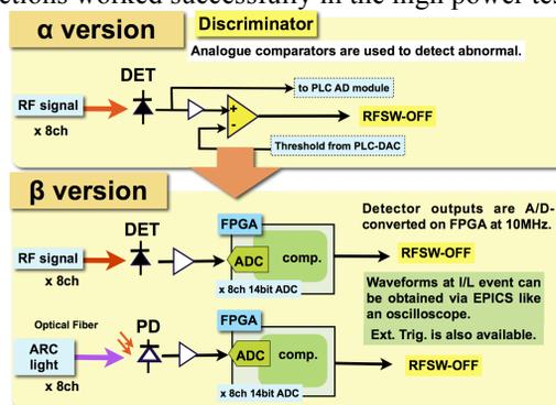
Figure 1: Main difference between the  $\alpha$  and  $\beta$ -version.
