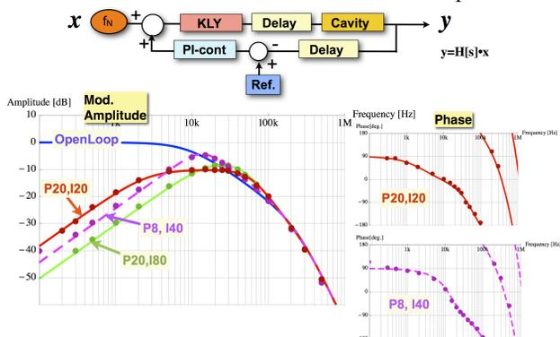
Figure 6: Bode plots of cavity response to disturbance inside the closed loop (e.g. DAC output noise).
