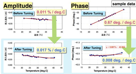
Figure 2: Fine-tuning of BPF temperature characteristics to improve thermal stability.
