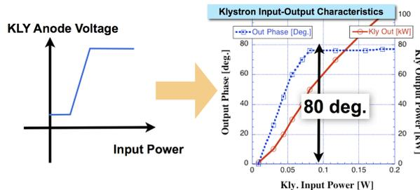
Figure 7: Klystron phase shift due to the anode voltage control.
