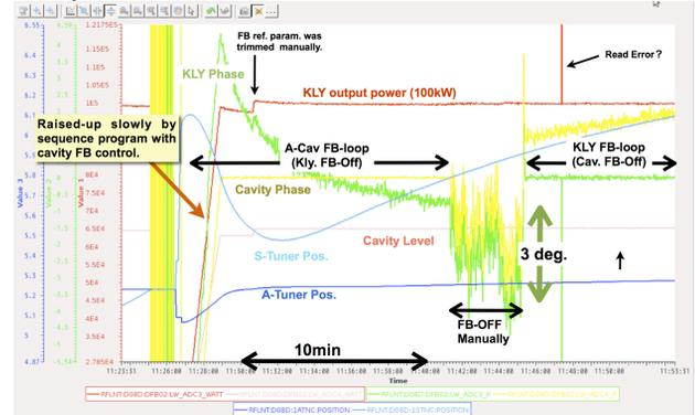
Figure 4: Strip chart of cavity power rising-up.
