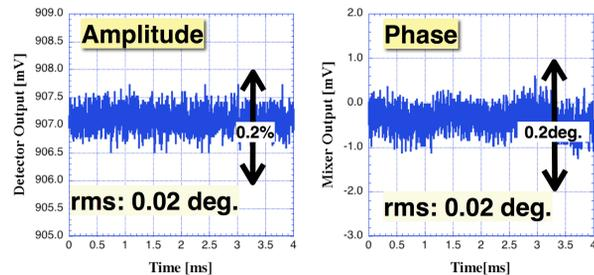
Figure 5: Short-term amplitude and phase stability under feedback control evaluated by out-of-loop measurement.
