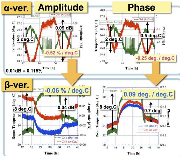
Figure 3: Measured thermal stability of the overall LLRF system. Trend graph for 2 days.
