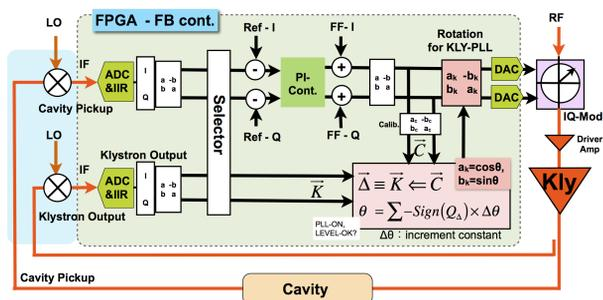
Figure 8: Design of klystron phase lock loop, which will be implemented in the FPGA.
