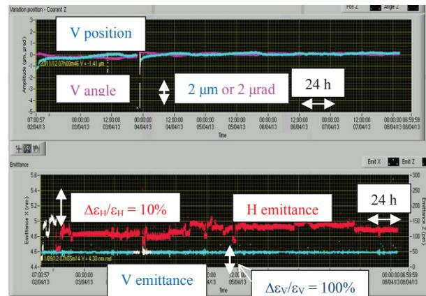
Figure 2: One week stability records of vertical position and angle as well as emittances for Anatomix BL. The white trace areas show beam times out of tolerance. The H emittance scale is much larger than the vertical one.
