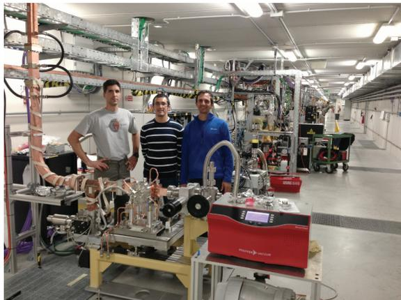
Figure 7: Fermi II gun installed in the test area (Fermi FEL tunnel).
