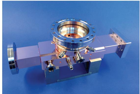
Figure 4: picture of the Fermi II Gun after final brazing.
