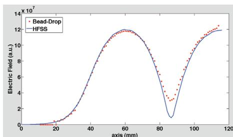
Figure 6: On-axis electric field profile. Data (red dots) and fit (blue line).
