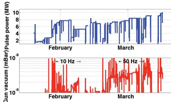
Figure 9: Monitoring of the high-power conditioning and vacuum levels.
