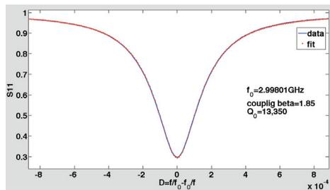
Figure 5: reflection coefficient. Data (red dots) and fit (blue line).
