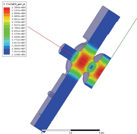
Figure 1: 3D model used for HFSS simulation. Surface electric field is shown.
