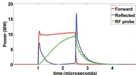
Figure 8: Power forms of the RF signals.
