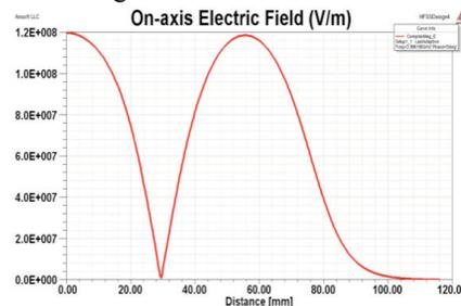
Figure 2: On-axis electric field, from HFSS.
