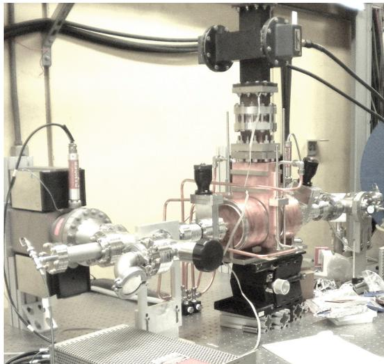
Figure 8: HGS structure installed at Livermore. Vacuum piping and cooling system are also shown.
