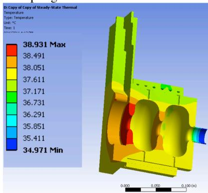
Figure 4: Temperature distribution inside the HGS.
