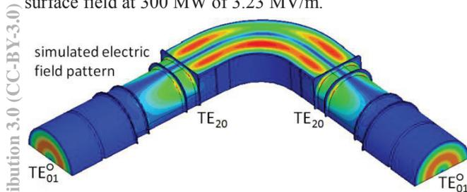
Figure 2: Half geometry of the circular TE<sub>01</sub> mode bend design with electric field patterns illustrating mode conversion in the interior.
