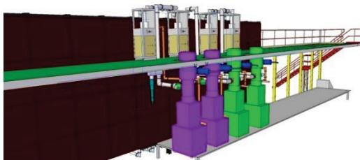
Figure 3: RF Amplifier chain, final installation plan.
