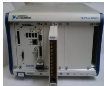
Figure 2: PXI express chassis with FPGA module.
