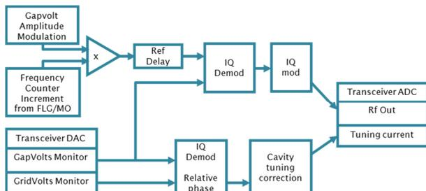
Figure 6: Cavity RF IQ loop and tuning loop implemented on a single FPGA module.
