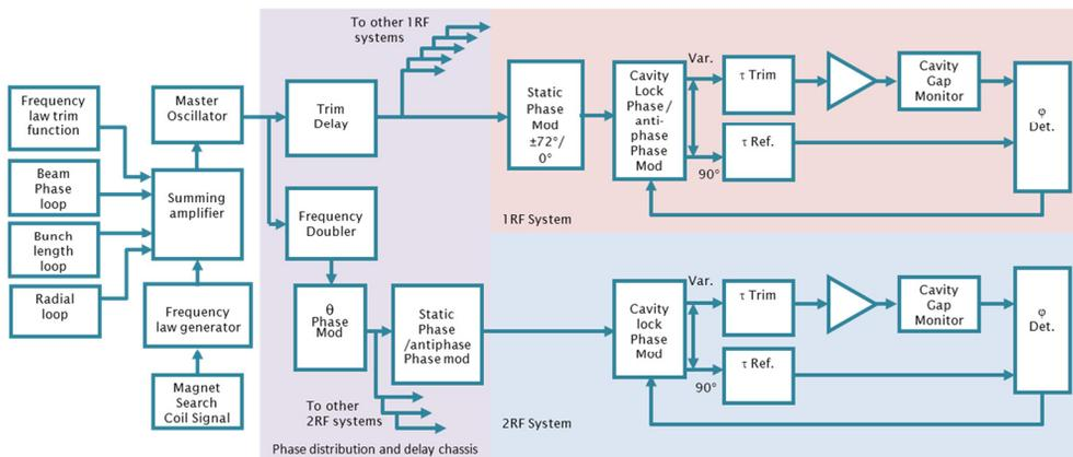
Figure 1: System diagram of the ISIS low power RF.
