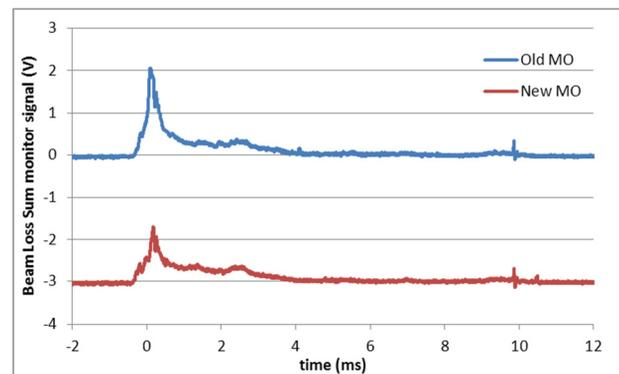
Figure 5: Typical beam loss monitor signals for the Old MO compared with the new FPGA MO (-3V offset).
