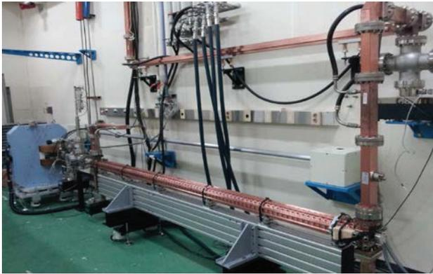
Figure 8 : Photo of the tunnel of the high power test facility for the accelerating structure (RI structure installed).
