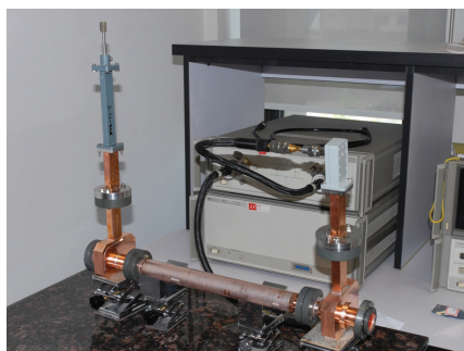
Figure 4: RF Measurement Setup after Brazing
