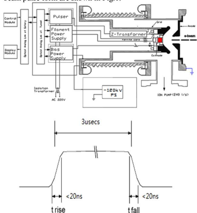
Figure 1: The gun structure (top) and the gun beam pulse form (bottom).
