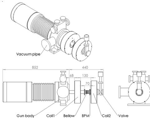
Figure 3: Element distributions between gun and bunching system.
