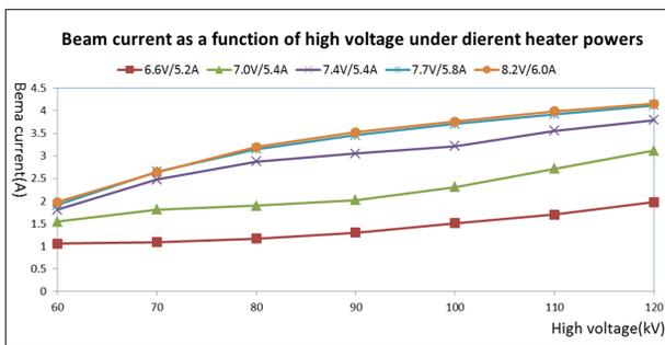
Figure 7: Beam current vs. high voltage.
