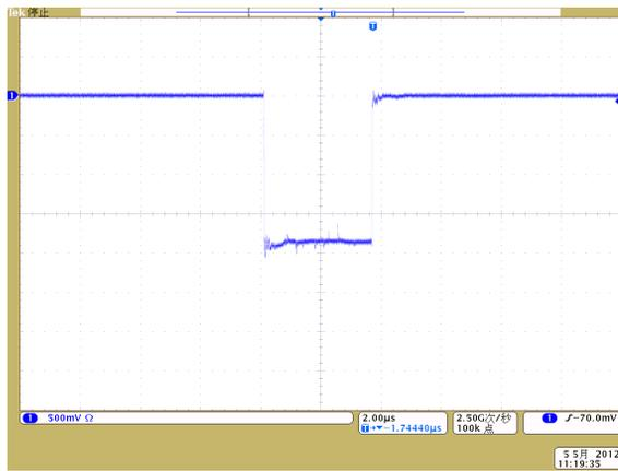
Figure 6: Gun current signal from oscilloscope.
