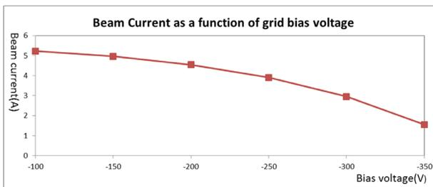
Figure 8: Beam current vs. grid bias voltage.
