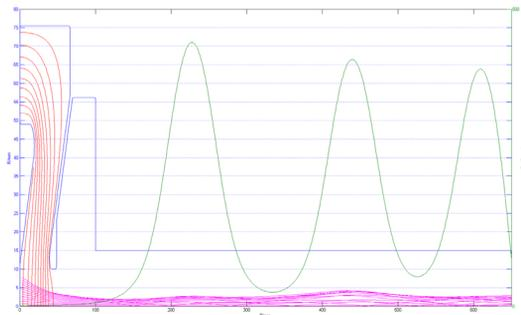
Figure 2: Beam optics with 2.0A/120kV in the gun.
