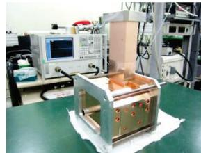
Figure 8: Photo of 2 cell rf-deflector cavity
