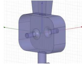
Figure 3: Single-cell structure of the rf-deflector.
