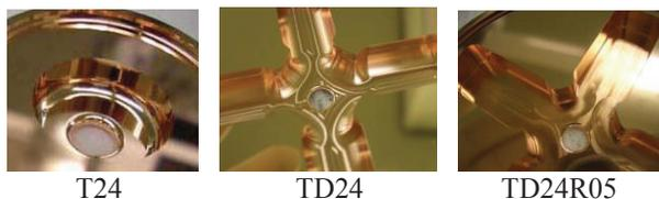
Figure 1: CLIC prototype structure cells.
