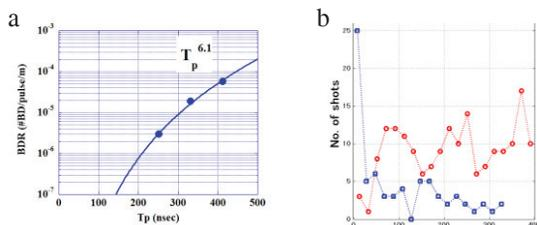
Figure 6: Breakdown characteristics of TD24R05#2. (a) BDR vs. pulse width and (b) breakdown timing distribution.
