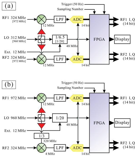
Figure 2: Block diagrams of the cavity phase monitors. (a) shows that for the dedicated 324-MHz [972-MHz] cavities. (b) represents that for the combined system of 324 MHz and 972 MHz.
