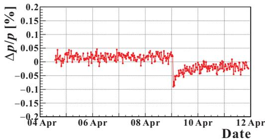
Figure 4: Trend chart of the momentum spread with FCTs. It was calculated from time of flight around the debuncher2 cavity.
