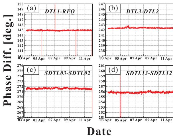
Figure 3: Trend Chart of the phase stability by the cavity phase monitors.
