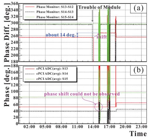
Figure 5: Recorded data for the SDTL13-15 sections in 24th May, 2013. The phase shift could not be seen with the measurement of (b) cPCI ADCs, but could be confirmed with that of (a) the cavity phase monitor.
