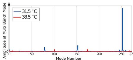
Figure 8: Multi bunch mode spectrum of a 30 mA beam at 1.2 GeV with different temperatures of the cavities.
