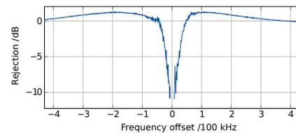
Figure 4: Optimized transfer function to the error point of the closed loop stabilization performance at 30 mA.
