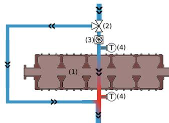
Figure 7: Variable water cooling bypass system of one PETRA cavity (1) with three-way valve (2), flow meter (3) and temperature sensors (4).
