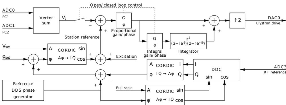
Figure 3: Principle of the LLRF’s open/closed loop RF field stabilization.
