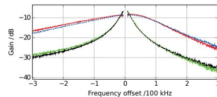
Figure 6: Transfer functions of PC1 open- (green) and closed loop (red), PC2 open- (black) and closed loop (blue).
