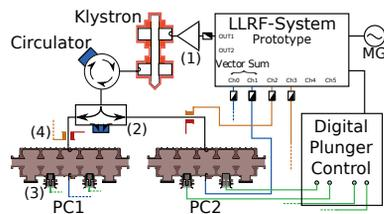
Figure 2: Integration of the LLRF system into the RF system: tuning plungers (3) and directional couplers (4).
