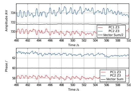
Figure 5: Closed loop performance with static set points.
