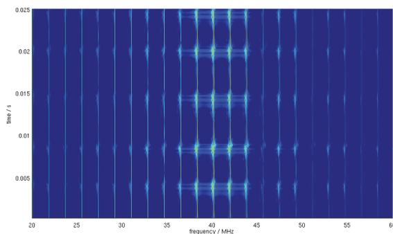
Figure 3: Waterfall plot of the beam spectrum.
