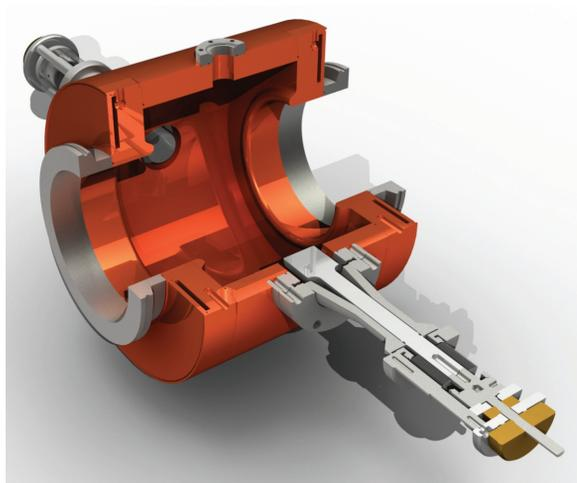
Figure 5: Cavity for narrow band feedback system optimized to the frequency of mode 253 being 1.46 GHz.
