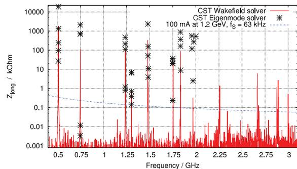
Figure 1: Wake impedance and natural damping calculations [3] of a five-cell PETRA cavity using CST Microwave Studio<sup>TM</sup>.
