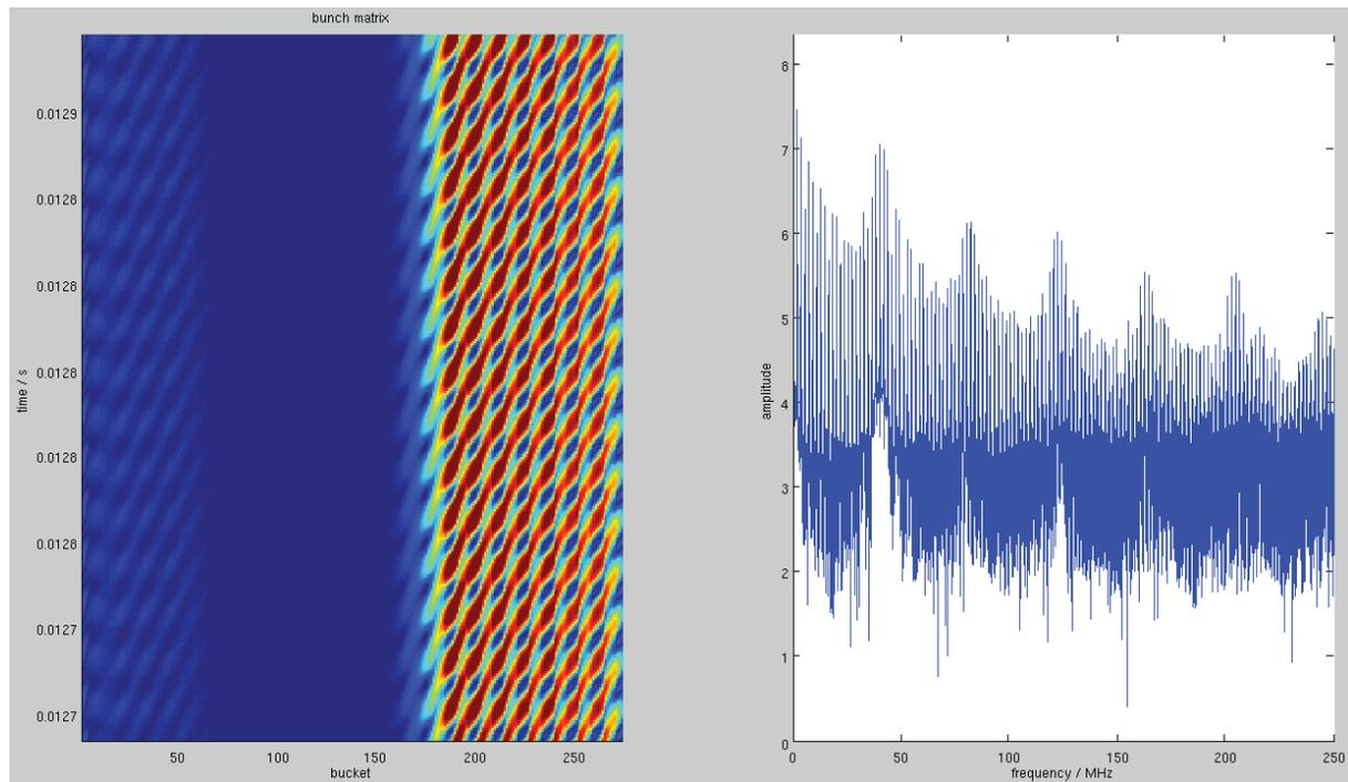
Figure 4: Time evolution and spectrum of the longitudinal phase space.
