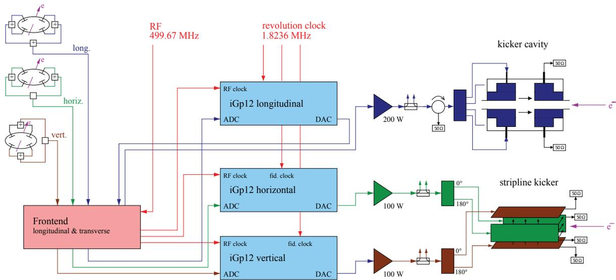
Figure 2: Overview of the bunch-by-bunch feedback system at ELSA [3].
