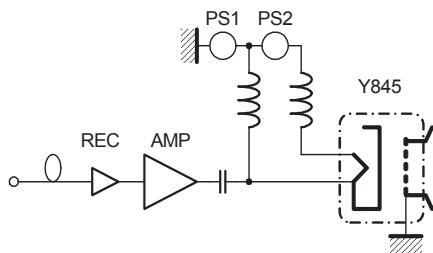
Figure 5: EIMAC – Y845 cathode's polarization scheme.
