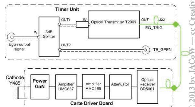
Figure 4: Electron Gun modulator.
