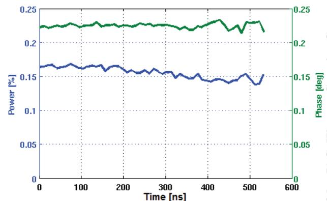
Figure 3: Residual pulse-to-pulse RF jitter along the pulse at the input of one accelerating structure.
