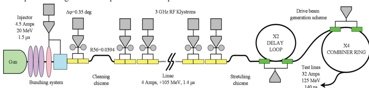
Figure 1: CTF3 drive beam layout.
