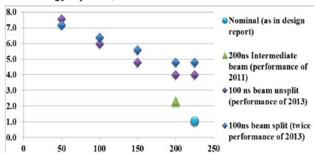
Figure 1: Expected peak luminosity ( $10^{27}$  Hz/cm<sup>2</sup>) at 7 ZTeV, with respect to batch spacing in the SPS (ns).
