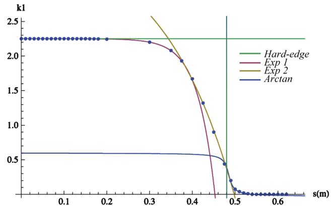
Figure 4: The exponential and arctan functions described in equation 3, combined as described in equation 4 and fitted to field data (circles).
