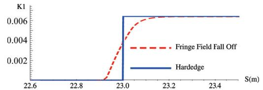
Figure 1: Hard-edge field compared to realistic falloff.
