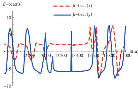
Figure 6:  $\beta$ -beat for HLLHCV1.0 IR 5 optics with  $\beta^* = 15$  cm.
