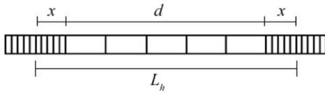
Figure 3: Example of one hard-edged magnet replaced by 5 central magnets and 10 “fringe” magnets, which are used to model a more accurate field falloff.
