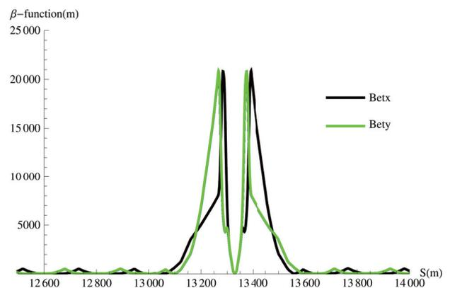
Figure 2:  $\beta$ -function in the HL-LHC optics in IR5 for  $\beta^* = 15 \text{ cm}$ .
