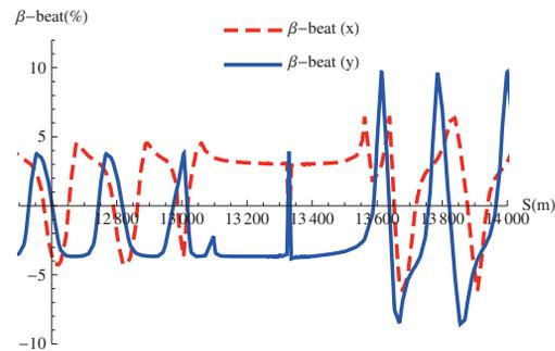
Figure 5:  $\beta$ -beat for SLHCV3.1b IR 5 optics with  $\beta^* = 15$  cm.
