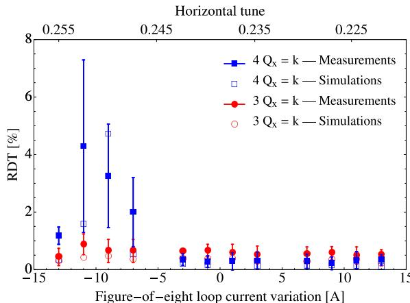
Figure 4: RDT vs. figure-of-eight loop current variation [A]
