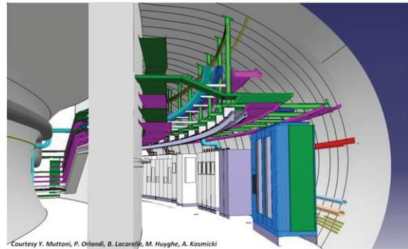
Figure 3: UL557 cross section after equipment relocation.
