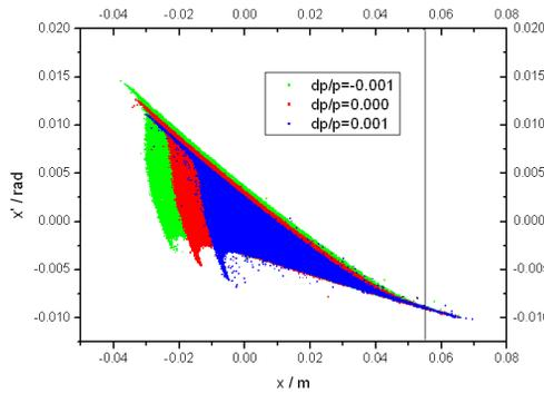
Figure 4: Separatrices of the extracted beam.
