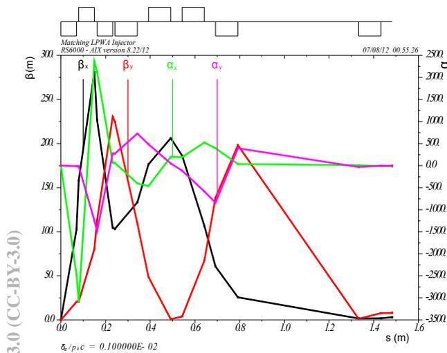
Figure 2: Exemplary transfer line, matching the LWFA generated bunches to the ANKA storage ring.
