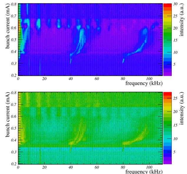
Figure 1: Spectra of THz radiation for different bunch currents measured directly with a spectrum analyzer (top) and indirectly using the FFT of an oscilloscope (bottom). The intensity changes at 0.37 and 0.72 mA are due to the attenuation change mentioned above. Both methods show the same bursting pattern and the line at  $f_s = 8.36$  kHz is present at all currents.
