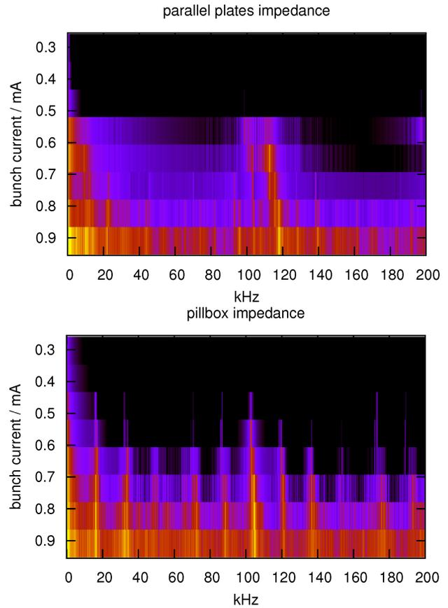
Figure 2: Simulated THz radiation spectra for different bunch currents using the parallel plates impedance (top) and the pillbox impedance (bottom) [7].
