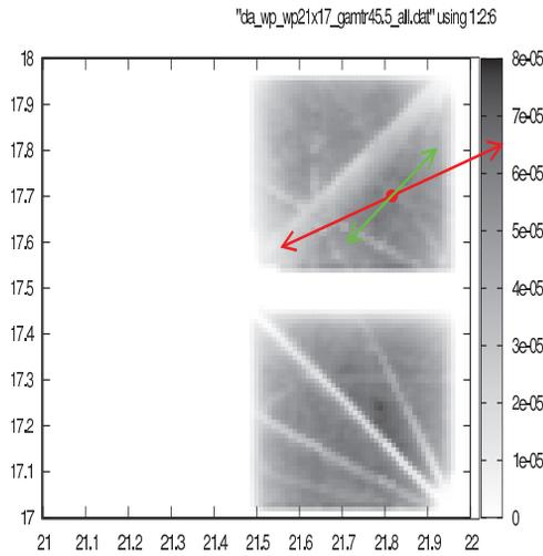
Figure 1: Dynamic aperture scan, working point and tune spread due to  $\delta = \pm 0.0043$  with natural chromaticity (red arrow) and reduced to  $\Delta Q_{x,max} = \Delta Q_{y,max} = \pm 0.1$  by correcting the chromaticities (green arrow) obtained for  $\gamma_{tr} = 45.5$ . The dynamic aperture was determined by tracking a single particle during 500 turns for different angles in the  $x - y$  plane. The results were averaged to obtain the dynamic aperture shown in this figure.
