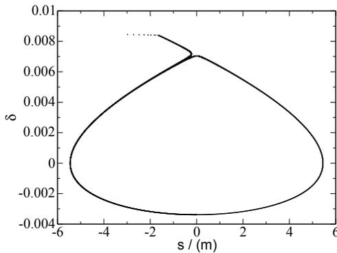
Figure 2: Stable and unstable longitudinal phase space trajectories close to the separatrix simulated for extraction conditions:  $E = 29$  GeV,  $\gamma_{tr} = 45.5$ ,  $V_{rf} = 300$  kV. The synchronous phase  $\phi_s = 0$  corresponding to constant energy and the lattice without magnet imperfections and chromaticity correction were used.
