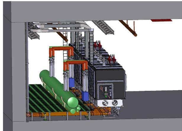
Figure 4: Schematic drawing of connections to a cryomodule through U-tubes with the helium distribution lines in the FRIB linac tunnel.
