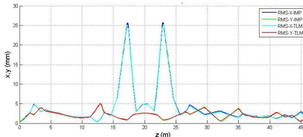
Figure 6: Beam envelop tracking with thin lens model (TLM) closely agrees with multi-particle tracking simulations using IMPACT (IMP) for multi charge state beams.
