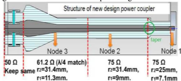
Figure 3: Multipacting free RF coupler for the HWR cavity.
