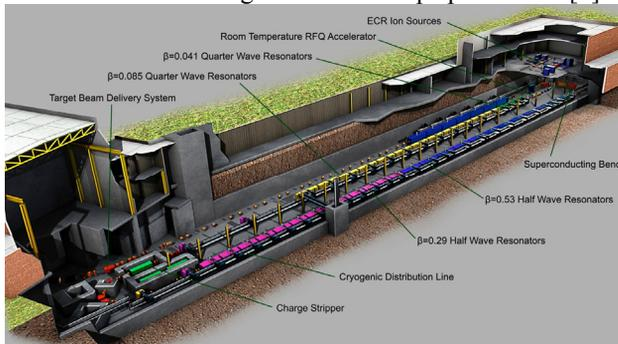
Figure 1: Layout the FRIB driver linac.
