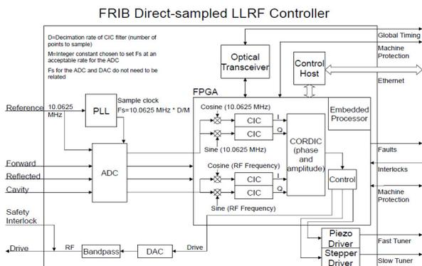
Figure 5: Block diagram of the FRIB LLRF controller.
