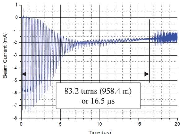
Figure 2: Measured current profile using the resistive wall current monitor, for the 6 mA 98.77 ns bunch with a fill factor of 0.5. Note the onset of the instability at 16.5  $\mu$ s.
