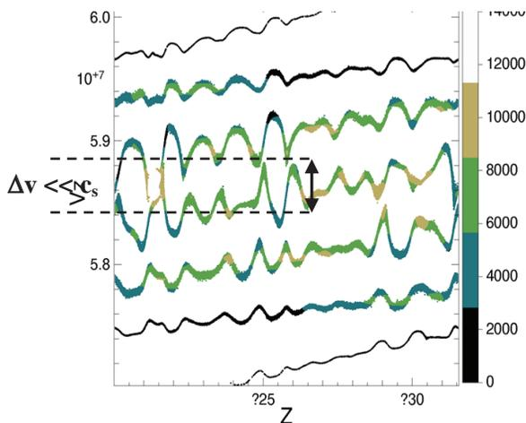
Figure 3: Simulated phase space image over multiple turns, wrapping the ring  $>6C$  for an injected bunch length of  $\Delta L = 0.506C$  or fill factor of 0.506. The length of the z axis corresponds to the ring circumference. This simulation includes no current loss.
