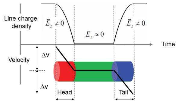
Figure 1: Illustration of the line-charge density and velocity profile of an intense rectangular bunch. Longitudinal space-charge accelerates/decelerates particles in both the head and tail of the bunch from the injected beam velocity,  $v_o$ .
