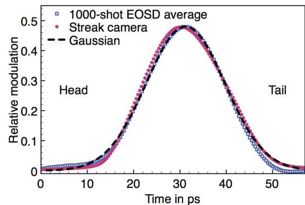
Figure 10: Averages of bunch profiles obtained from streak camera measurements and from single shot profile acquisitions with the electro-optical spectral decoding method. The smooth average shapes of both methods are similar [31].
