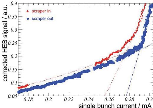
Figure 6: Time averaged amplitude of the THz signal measured with a NbN detector system as a function of the single bunch current with and without a scraper positioned close to the beam at ANKA. The dashed lines represent fits to the steady state and bursting regimes, respectively. The crossing points can serve as an estimate for the bursting threshold [27].
