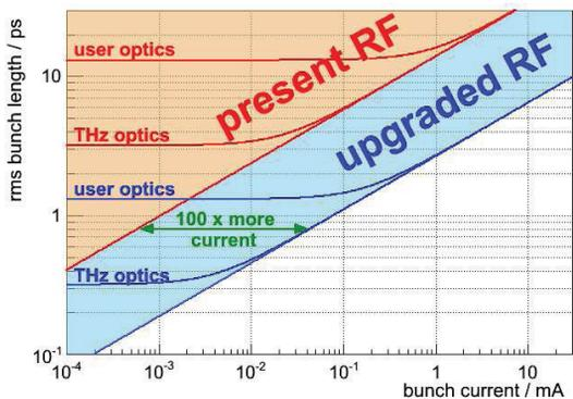
Figure 4: Bunch length as a function of bunch current at BESSY II for the present situation and with a 100 time stronger RF gradient [8].
