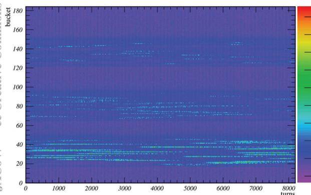
Figure 8: Quasi-simultaneous measurement of THz signals from all bunches in the ANKA storage ring measured with an ultra-fast YBCO detector and dedicated DAQ system [24, 29, 30]. The bursting signature is clearly visible in all three trains.
