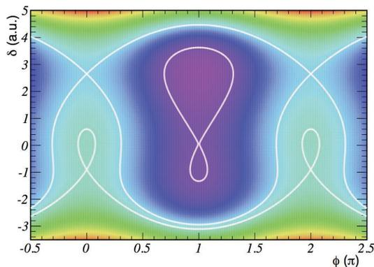
Figure 2: Nonlinear longitudinal phase space with alpha buckets (see [7] for a detailed description).
