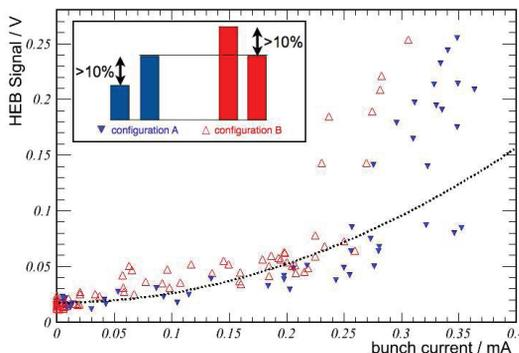
Figure 7: THz signal from a NbN detector for the individual bunches of a multi-bunch filling pattern at ANKA. The colour coding represents the current ratio of the leading bunch to its successor. The dashed curve is a global fit to all data points below the bursting threshold. The earlier onset of the bursting and the higher steady state power are clearly visible [27].
