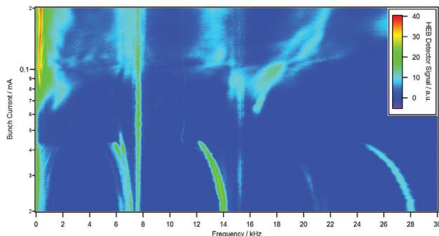
Figure 5: Spectrogram of the turn-by-turn THz signal measured with the HEB detector system at ANKA as a function of the single bunch current [24].
