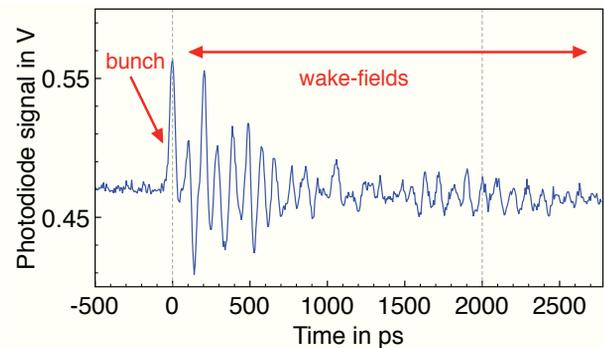
Figure 9: Electro-optical sampling measurement of the electric field induced birefringence inside a GaP crystal from a passing electron bunch inside the ANKA vacuum chamber [31].
