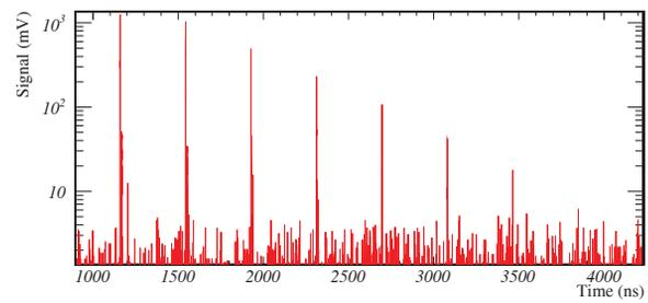
Figure 3: Laser-induced THz radiation recorded with a HEB detector system over about 10 revolutions at the DELTA a 1.5 GeV synchrotron light source at TU Dortmund [12].
