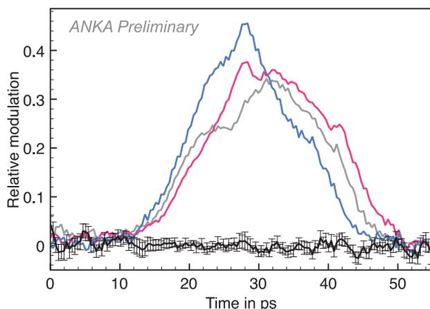
Figure 11: Single shot measurements recorded with the electro-optical spectral decoding method (coloured curves) within a few seconds. The black line correspond to the average of 100 background acquisitions. The error bars reflect the standard deviation of these data sets. The single shot measurements exhibit significantly different bunch shapes and structures (Courtesy N. Hiller, see also [31] for more details).
