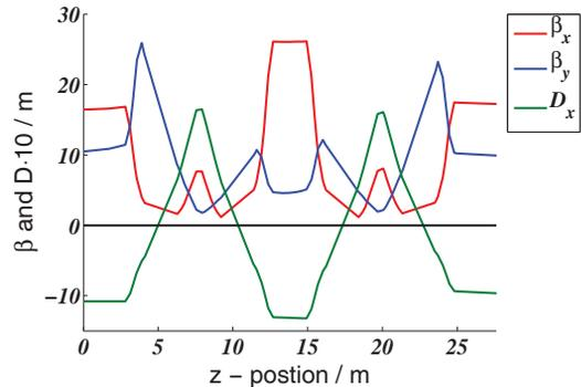
Figure 1: Example of betatron functions and horizontal dispersion of the low alpha optics or one of four sectors of the ANKA storage ring with an  $\alpha_c$  of  $4.6 \cdot 10^{-4}$ .
