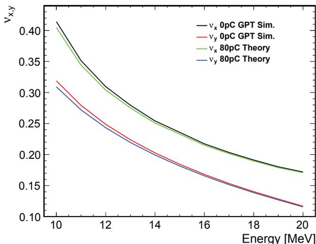
Figure 5: Theoretical tune shift from an 80 pC bunch-charge, compared with the tune calculated from GPT simulations with 0 pC.
