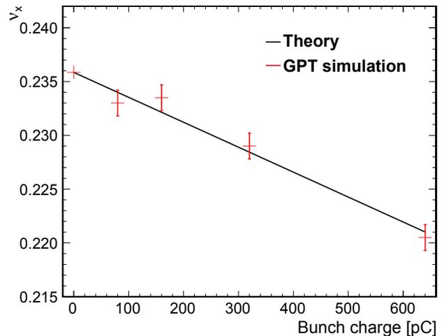
Figure 6: A demonstration of tune shift caused by space-charge over a range of bunch-charges (within and beyond the EMMA regime), with a fixed beam energy of 15 MeV. The theoretical data is taken with respect to the 0 pC simulation as performed by GPT, with no uncertainty on this data point.
