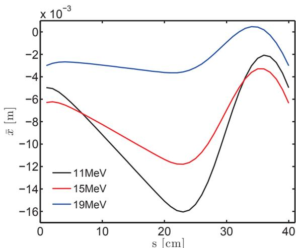
Figure 3: Mean horizontal position for three closed orbits of differing energy in one EMMA cell. The transverse coordinates at the entrance of the cell are equal to those at the exit after a rotation of  $2\pi/42$ , not represented in this figure.
