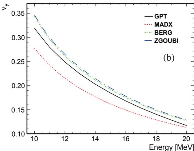
Figure 4: Comparison of the a) horizontal, and b) vertical tune produced by different codes modelling the EMMA ring with baseline parameters.
