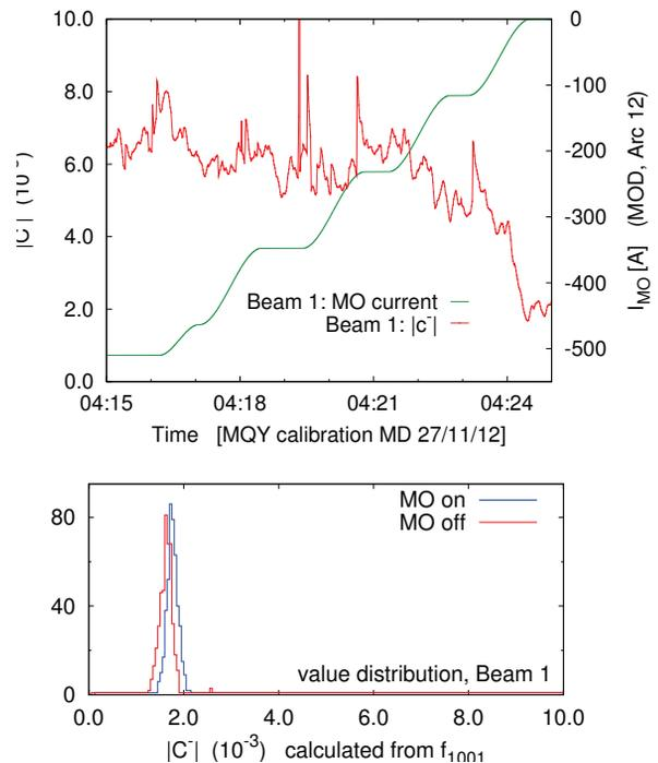
Figure 2: BBQ (upper plot) and RDT (lower plot) shifts on depowering the MO during November 2012.
