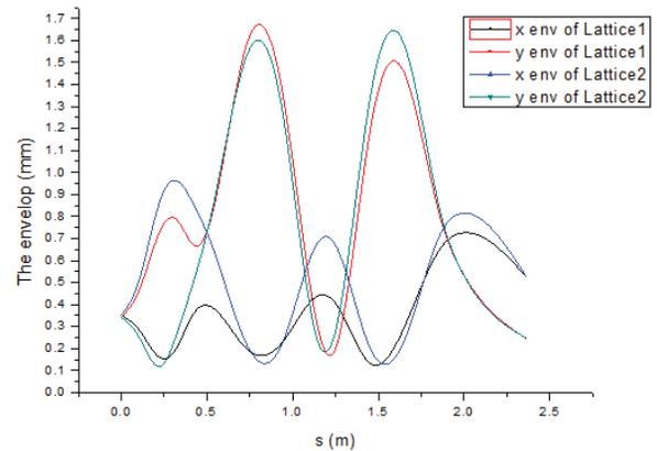
Figure 3: The envelope of the beams with different lattices.
