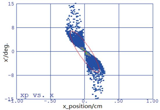
Figure 4: Phase-space plot at the entrance of the linac.
