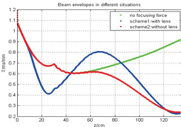
Figure 3: Beam envelopes in three different situations.
