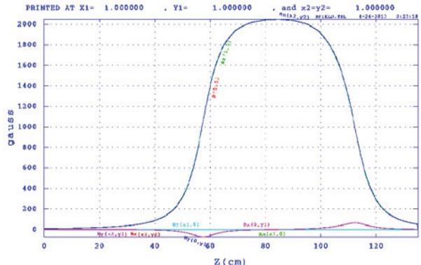
Figure 5: Magnetic field distribution of scheme 2.
