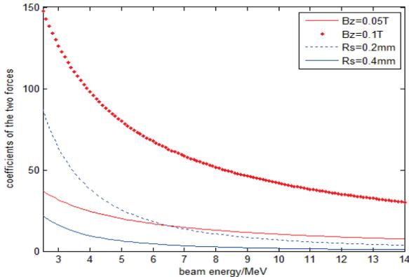
Figure 2: Coefficients of the two forces vary with the beam energy.
