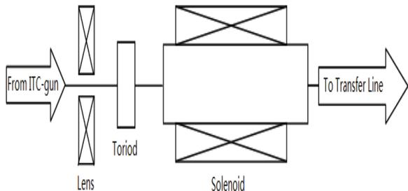
Figure 1: Focusing system for the linac.
