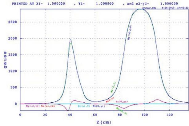
Figure 7: Magnetic field distribution of scheme 3.
