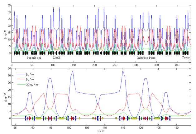
Figure 1: Linear optics along the SSRF storage ring and its double-mini- $\beta_v$  optics (DMB: Double-Mini-Betay).
