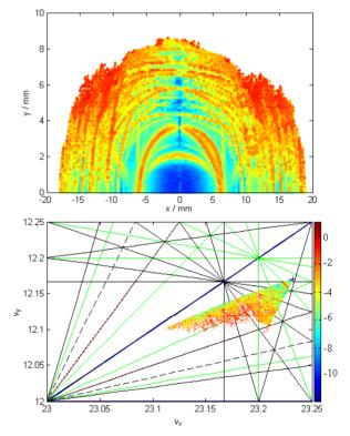
Figure 3: Dynamic aperture and frequency maps of on-momentum particle in the SSRF storage ring.
