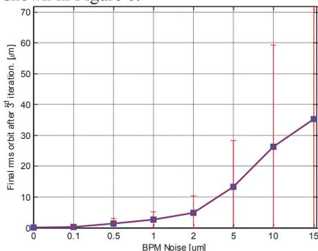
Figure 6: Influence of BPM resolution/noise to the final orbit.
