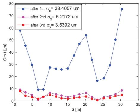
Figure 5: The mean rms orbit at 900MeV in each iteration.
