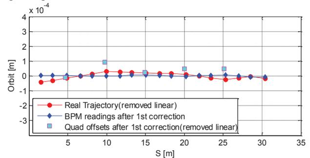
Figure 3: The absolute orbits (removed linear component), BPM readings and quadrupole offset after 1<sup>st</sup> iteration.
