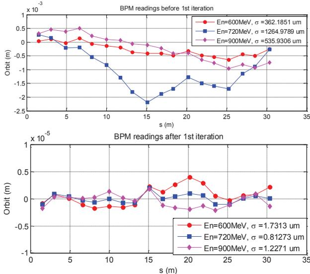
Figure 1: BPM readings before and after 1<sup>st</sup> iteration.
