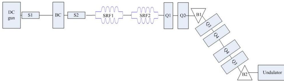
Figure 1: Block diagram of the CAEP FEL-THz facility. S1 and S2 are solenoidal lenses. BC is the RF Buncher Cavity. SRF1 and SRF2 the superconducting RF Cavities, Q1, Q2, Q3 and Q4 are quadrupoles, B1 and B2 are dipoles.
