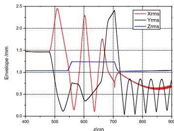
Figure 5: Evolution of beam size and bunch length in achromatic section and wiggler.
