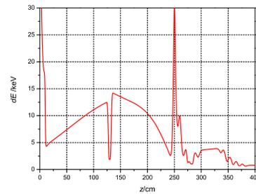
Figure 4: Evolution of bunch rms energy spread.
