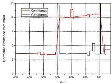
Figure 6: Evolution of Beam normalized RMS transverse emittance in achromatic section.
