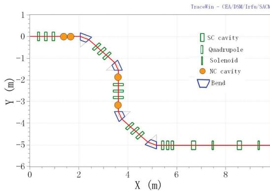
Figure 1: The layout of MEBT2 line for injector-1.
