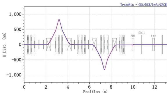
Figure 2: The dispersion function along the MEBT2 line.
