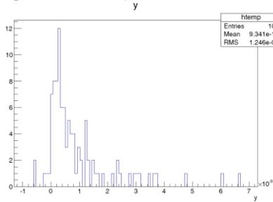
Figure 2: Orthogonality check of  $\alpha_x$  knob when introducing gradient errors 1e-3.
