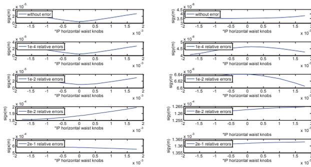
Figure 1:  $\sigma_x$  and  $\sigma_y$  dependence on the  $\alpha_x$  knob with and without gradient errors.
