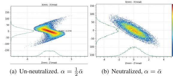
Figure 3: Horizontal phase space at the RFQ input.
